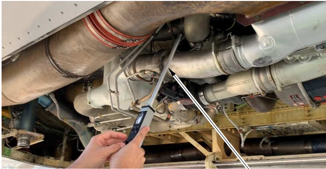
AIR CONDITIONING CHECK (EXAMPLE)
