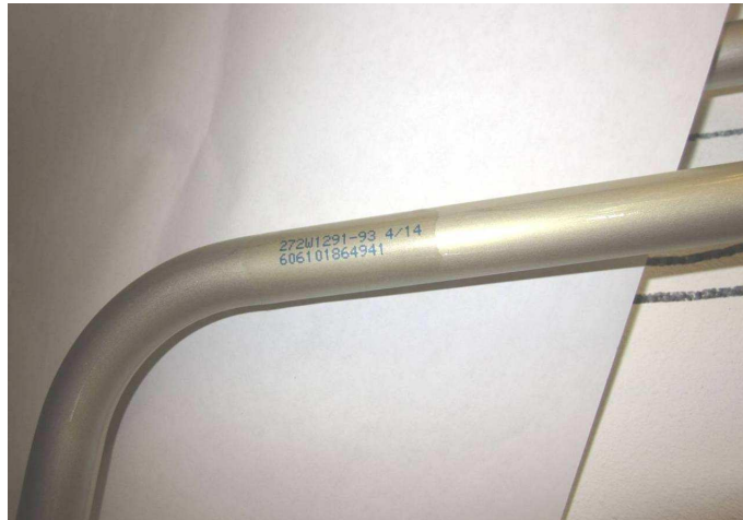
EXAMPLE OF ALUMINUM TUBE (PART NUMBER IS RUBBER STAMPED WITH CLEAR OVERCOAT ON TUBE)
