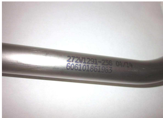
EXAMPLE OF TITANIUM TUBE (PART NUMBER IS ELECTRO-ETCHED ON TUBE)
