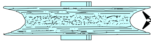
PULLEY NOT ALIGNED CORRECTLY
