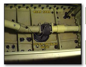
Bonded valve inside the tank
