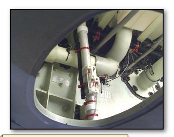
Electrical harnesses in the tanks use very low voltage current (less than 5 VDC) and are far enough for the surrounding equipment and structure (segregated routing).
