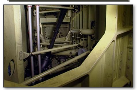
**EXAMPLE OF AN AIRBUS A330/A340 WING FUEL TANK (COLLECTOR CELL)**
