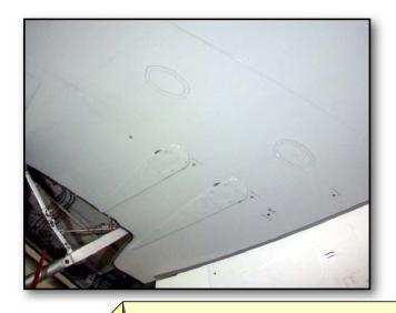
Fuel pumps are the only electrical equipment using high power current (115 VAC). Consequently, pumps harnesses are located under the lower wing skin panels outside the fuel tanks.
