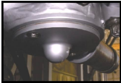
FWD JACKING DOME
