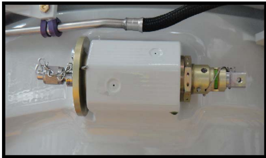
MLG OIL CHARGING VALVE AND CHANGEOVER VALVE
