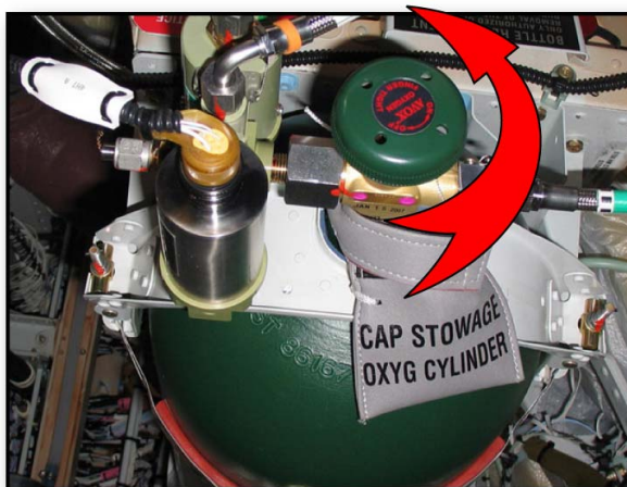
QUICK OPENING = OXYGEN OVERHEATING
