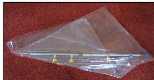
PUT EACH PIPE IN A SEALED VINYL BAG
