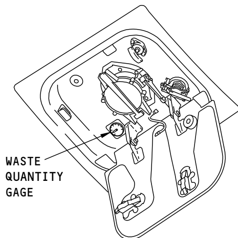
WASTE SERVICE PANEL
