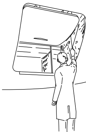
LOWER THE DOOR WITH BUNGEE LANYARD
