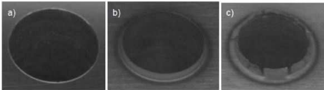
UNUSUAL BURRS (B AND C) IN COMPARISON WITH A BURR AFTER DRILLING IN REFERENCE CONDITIONS (A) (EXAMPLE)
