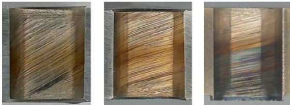
COLORING FOR DIFFERENT DEGRADED CONDITIONS IN THE DRILLING OF INCONEL 718 (EXAMPLE)
