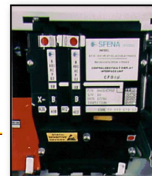
Centralized Fault Display Interface Unit (CFDIU)
