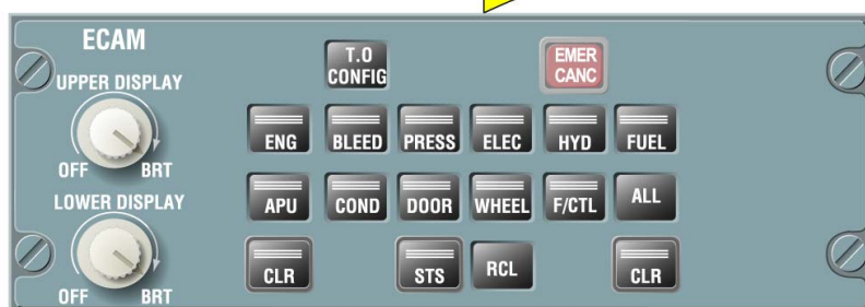
ECAM CONTROL PANEL (11VU)
