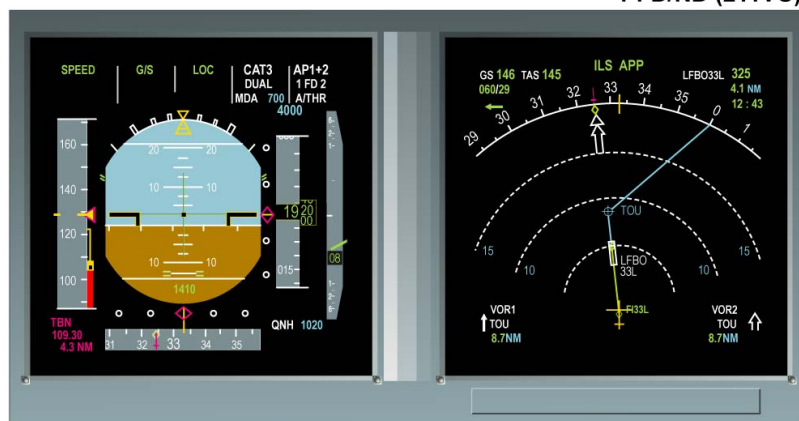
PANEL LOCATION/CONTROL AND INDICATING - EFIS DISPLAYS
