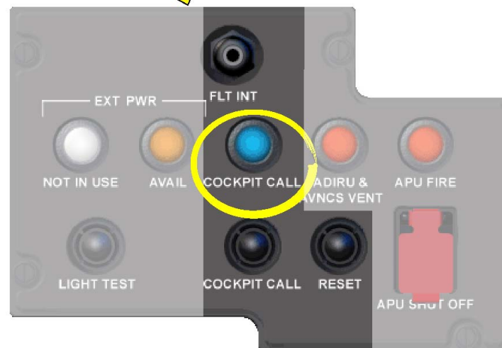
EXTERNAL POWER CONTROL PANEL (108VU)
