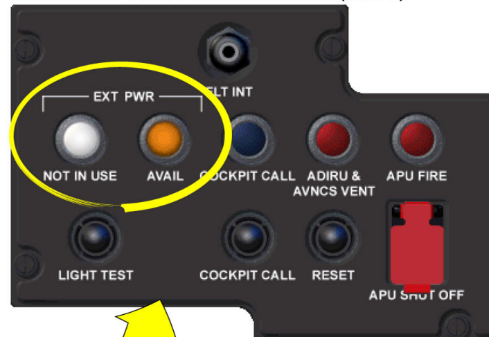
EXTERNAL POWER CONTROL PANEL (108VU)
