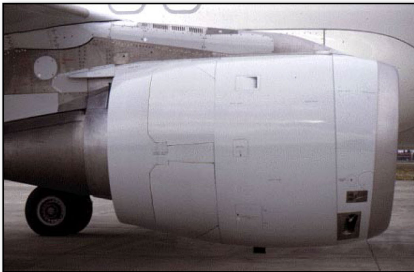
THRUST REVERSERS STOWED -PIVOTING BLOCKER DOORS CLOSED-
