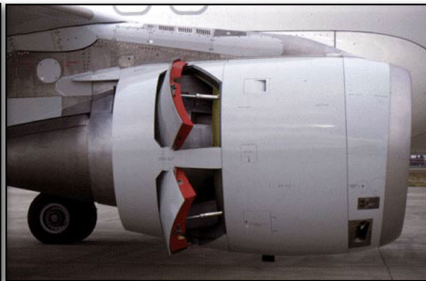
THRUST REVERSERS DEPLOYED -PIVOTING BLOCKER DOORS OPEN-
