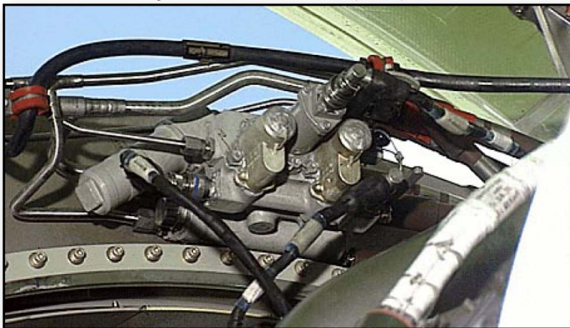
Hydraulic Control Unit (HCU)
